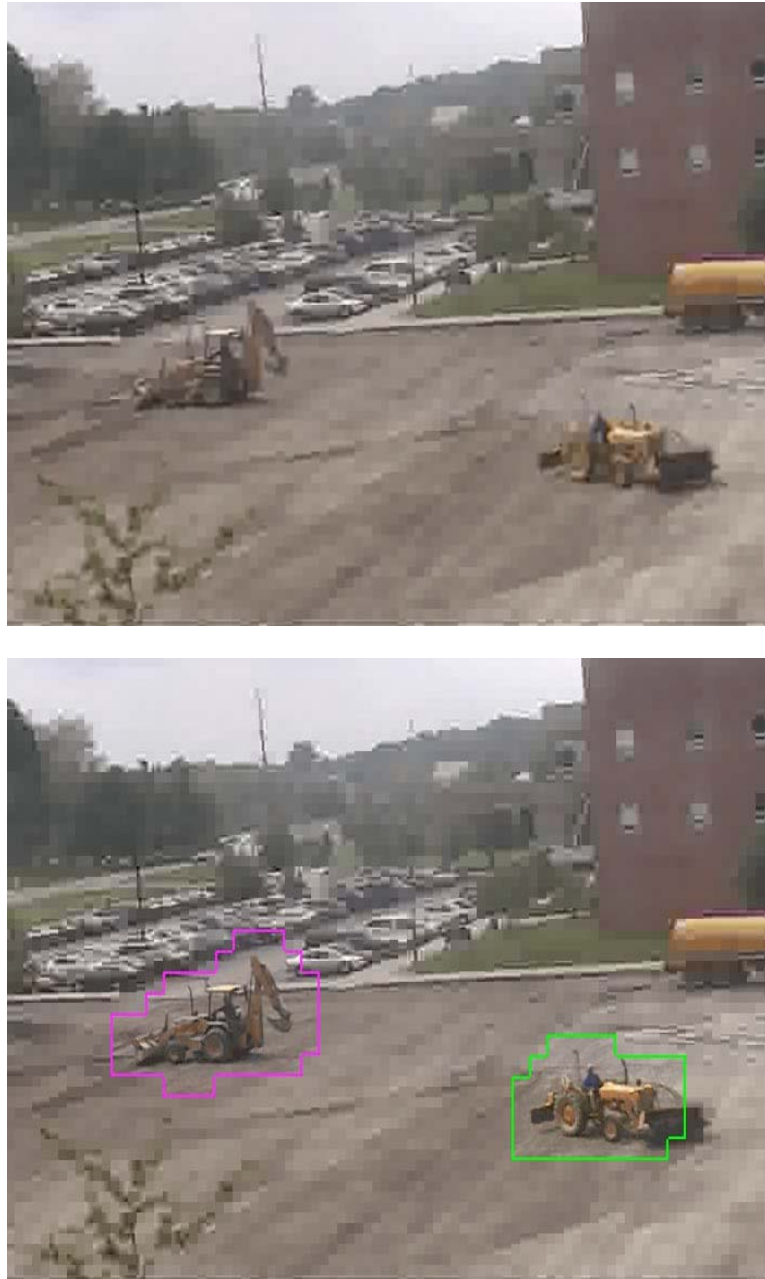
Figure 5.6 Perceptual quality comparison between non-object-based (upper) and object-based quality transcoding. In object-based transcoding, the two objects indicated by the color window have higher quality than in the non-object-based transcoding.
